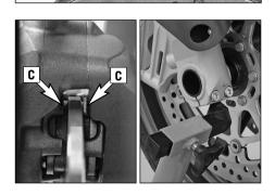
Take the left [4] and right distance bushing out of the shaft seal rings.
