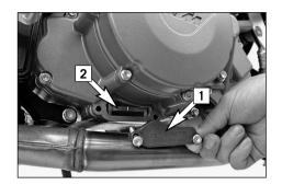
Mount the oil drain plug on the engine with a new seal ring and tighten to 20 Nm.
