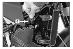
Unscrew the plug **[4]** and refill engine oil. Wait 20 seconds and check the oil level again. The quantity of oil between the MIN and MAX marks is 0.3 liter. Mount the plug and check the engine for leaks.
